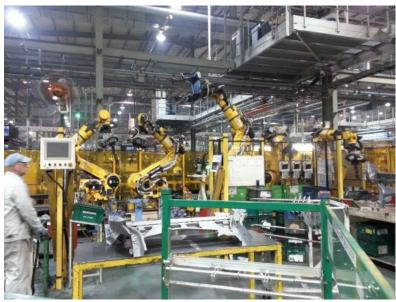
an array of different car parts. Whilst dodging forklift trucks and wearing some fetching yellow caps we watched the presses and robotic welders shape and join pieces of steel at an impressive speed.
